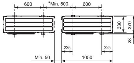
\* When installing a single outdoor unit, the clearance is 15 mm or more.
