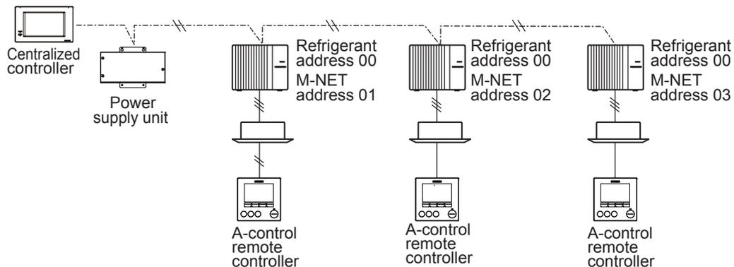
It is acceptable if M-NET wire (non-polar, 2-cores) is arranged in addition to the wiring for A-control.
