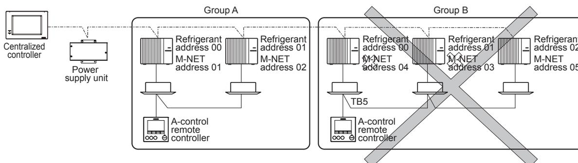
Note: In group B, M-NET address of the outdoor unit whose refrigerant address is "00" is not set to the minimum in the group. As "3" is right for this situation, the setting is wrong. Taking group A as a good sample, set the minimum M-NET address in the group for the outdoor unit whose refrigerant address is "00".
