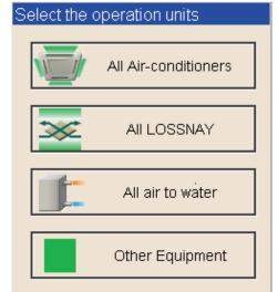
(2) After you have made the settings on the screen for batch operation, click [OK] and only the items for which operation was performed will be sent to all the air conditioner, ventilator (LOSSNAY) groups, Air To Water (PWFY) groups or general equipment groups.
