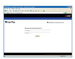
(4) If the security alert has not been disabled, after entering the web address and hitting the Enter (Return) key, a security alert message will alert asking if you want to proceed. This is because the AG-150A uses the self-authentication system. Click [Yes] and proceed.
