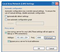
(6) Enter the IP address for the AG-150A (e.g. 192.168.1.1) in the Exceptions field of the Proxy Setting dialog and click the [OK] button to close the dialog and then close the other open dialogs to complete the setting.
