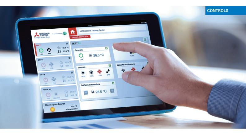
**Remote Monitoring Interface (RMI)** allows remote monitoring of up to 2,100 M Series, Mr Slim, City Multi, Lossnay and Commercial Heating (CAHV / CRHV) indoor units.
