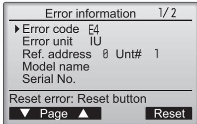
Error code, error unit, refrigerant address, unit model name, and serial number will appear.
