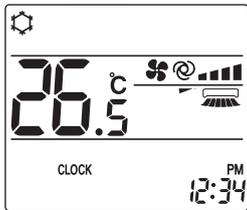
① Each time is pressed during operation, the setting changes in the following order: OFF → Direct → Indirect.
