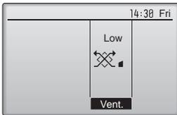
Press the [F3] button to go through the ventilation setting options in the order of "Off", "Low", and "High". \* Settable only when LOSSNAY unit is connected.
