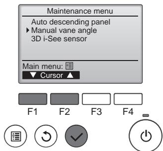
② Select "Manual vane angle" with the [F1] or [F2] button, and press the [SELECT] button.
