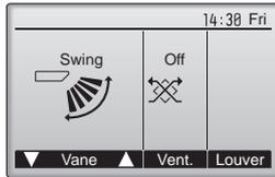
Press the [F1] or [F2] button to go through the vane setting options: "Step 1", "Step 2", "Step 3", "Step 4", "Step 5", "Swing" and "Auto". Select the desired setting.
