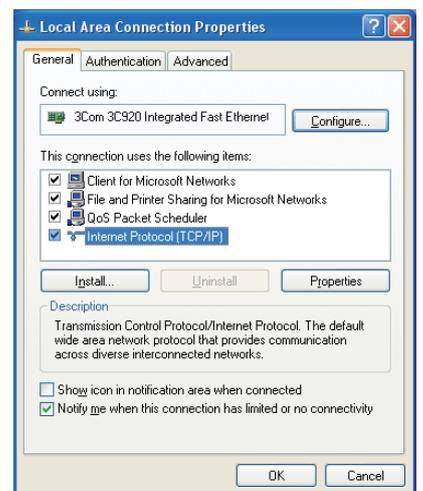
(4) In the [Internet Protocol (TCP/IP) Properties] dialog, click [Use the following IP address] and enter the IP address (for example, “192.168.1.101”) that you want to set in the IP address field. You normally set [255.255.255.0] as the subnet mask.
