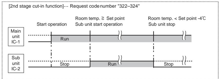
**11-1-2. How to set rotation function(Back-up function, 2nd stage cut-in function)**
