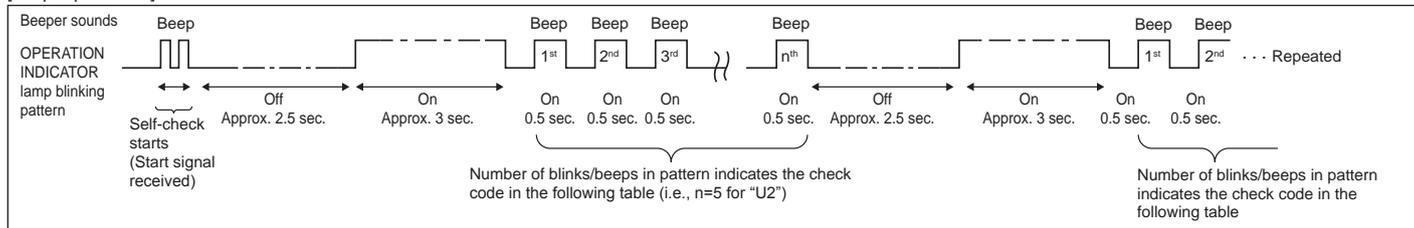
[Output pattern A] Errors detected by indoor unit
