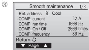
The Compressor-Accumulated operating (COMP. run) time is 10-hour unit, and the Compressor-Number of operation times (COMP. On/Off) is a 100-time unit (fractions discarded)
