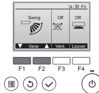
Press the [F1] or [F2] button to go through the vane setting options: "Auto", "Step 1", "Step 2", "Step 3", "Step 4", "Step 5" and "Swing". Select the desired setting.
