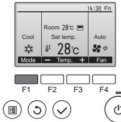
Press the [F1] button to go through the operation modes in the order of "Cool", "Dry", "Fan", "Auto", and "Heat". Select the desired operation mode.
