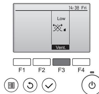
Press the [F3] button to go through the ventilation setting options in the order of "Off", "Low", and "High".
