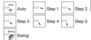
Select "Swing" to move the vanes up and down automatically. When set to "Step 1" through "Step 5", the vane will be fixed at the selected angle.
