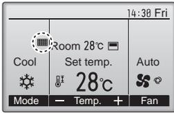
The filter icon will appear on the Main display in the Full mode when it is time to clean the filters.
