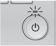
Press the [ON/OFF] button. The ON/OFF lamp will light up in green, and the operation will start.
