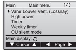
Select "Vane-Louver-Vent. (Lossnay)" from the Main menu, and press the [SELECT] button.
