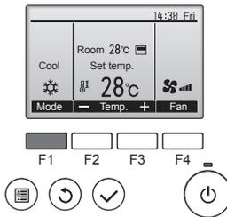
Press the [F1] button to go through the operation modes in the order of "Cool", "Dry", "Fan", "Auto", and "Heat". Select the desired operation mode.
