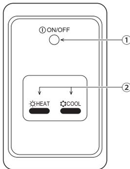
① **ON/OFF lamp** (lit when unit is operating; unlit when unit is not operating)
