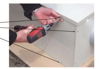
Slide the panel down and away to expose access to the Lossnay services.
