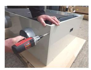
Place the top cover 1 over the housing panels and fix using 8 x M4 X 16 set screws 12 and 8 x nylon washers 10
