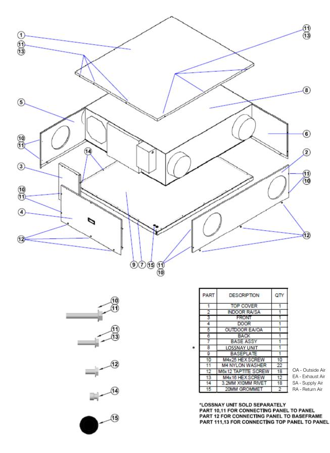
1 Carefully remove all housing parts from the packaging and place the base assembly consisting of parts (7,9,14,15) on a flat surface.
