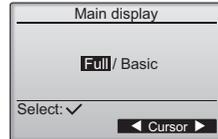
Note: This setting is only for the Main display. In the Basic mode, icons that indicate control status on timer and schedule settings will not appear on the display. Vane, louver, and ventilation settings or room temperature will not appear, either.
