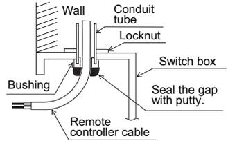
To reduce the risk of electric shock, malfunctions, or fire, seal the gap between the cables and cable access holes with putty.
