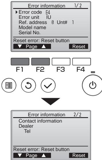
Error code, error unit, refrigerant address, unit model name, and serial number will appear. The model name and serial number will appear only if the information have been registered.
