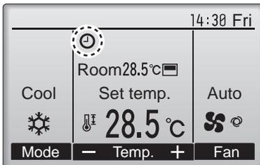
will appear on the Main display in the Full mode when the On/Off timer is enabled.
