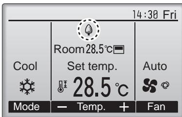
will appear on the Main display in the Full mode when the unit is operated in the energy saving mode.
