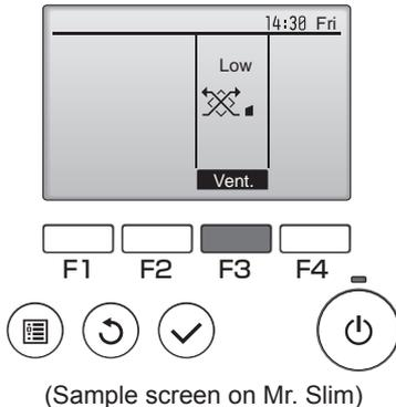
Press the **F3** button to go through the ventilation setting options in the order of "Off," "Low," and "High."
