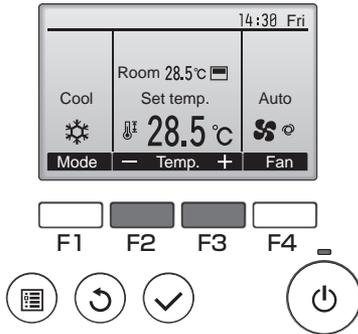
Press the **F2** button to decrease the preset temperature, and press the **F3** button to increase.
