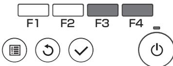
Adjust the contrast with the **F3** or **F4** button, and press the **MENU** or **RETURN** button.
