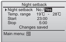
Move the cursor to the desired item with the **[F1]** or **[F2]** button out of Night setback No (disable)/Yes (enable), Temp. range, Start time, or Stop time. Change the settings with the **[F3]** or **[F4]** button.
