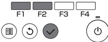
Move the cursor to the "Contrast" with the **F1** or **F2** button, and press the **SELECT** button.
