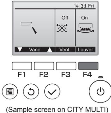
Press the **F4** button to turn the louver swing ON and OFF.
