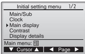
Move the cursor to the "Main display" with the **F1** or **F2** button, and press the **SELECT** button.
