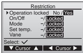
The screen to make the settings for the operation lock function will appear.
