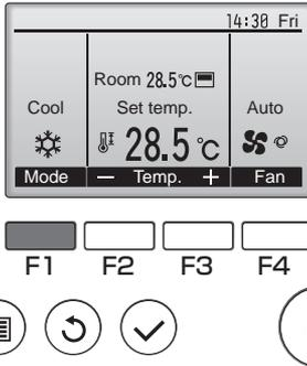
Press the **[F1]** button to go through the operation modes in the order of "Cool, Dry, Fan, Auto, and Heat." Select the desired operation mode.
