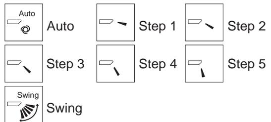
Select "Swing" to move the vanes up and down automatically.
