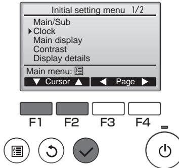
Move the cursor to the "Clock" with the **F1** or **F2** button, and press the **SELECT** button.
