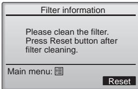
Press the **F4** button to reset filter sign.
