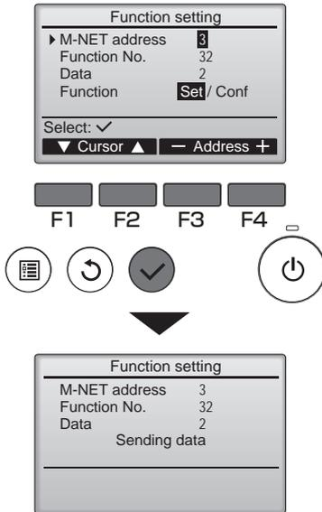
The Function setting screen will appear. Press the **F1** or **F2** button to move the cursor to one of the following: M-NET address, function setting number, or setting value. Then, press the **F3** or **F4** button to change the settings to the desired settings.
