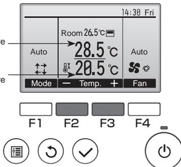
The current preset temperatures will appear. Press the **F2** or **F3** button to display the Settings screen.
