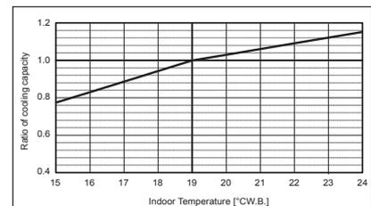
Figure 1 Indoor unit temperature correction
