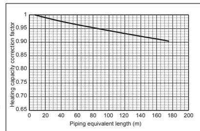
Figure 6 Correction of refrigerant piping length
