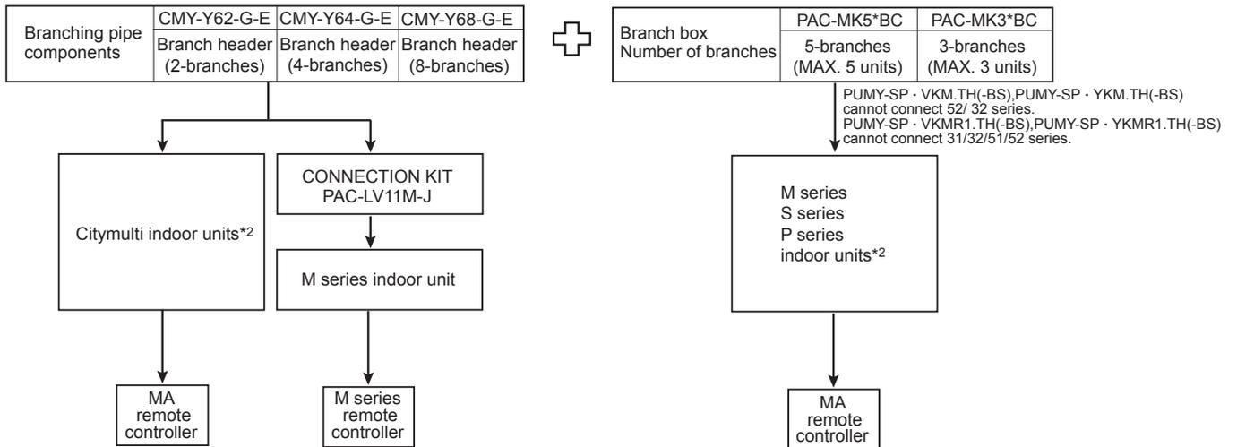
\*1 When connecting 7 indoor units via branch box, connectable citymulti indoor units are 3; connecting 8 indoor units via branch box, connectable citymulti indoor units are 2.
