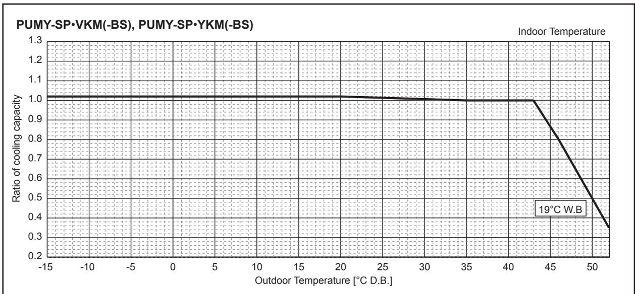
**Figure 9 Outdoor unit temperature correction**
