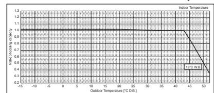
Figure 2 Outdoor unit temperature correction
