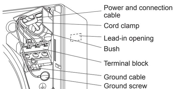
Operation requires a control switch. Have a control switch ready and connect the wiring shown in bold on the connection diagram below. Suitable cables:  $\varnothing 0.5$  to  $\varnothing 2.0$  mm diameter
