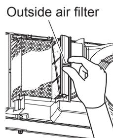
[3] Remove the outside air filter from the filter frame.
