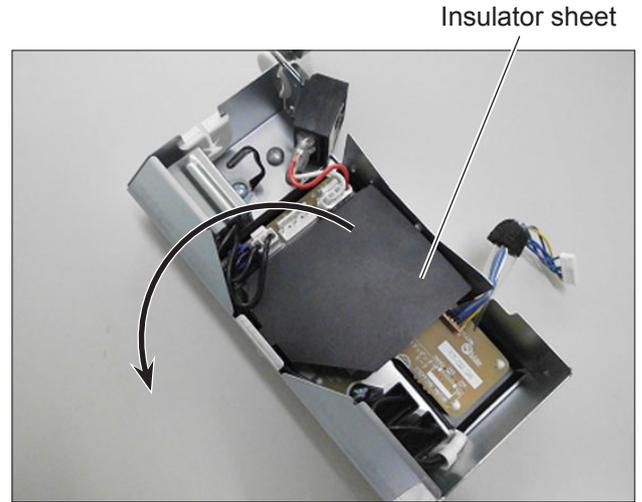
[4] Remove the rivets (six pieces, indicated by ○), and remove the main circuit board (VL-36M).
