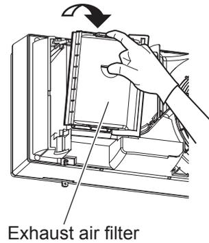
[2] Hold the knob of the outside air filter to pull it out, and remove it from the main unit.
