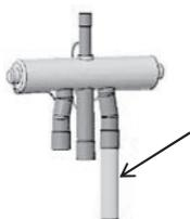
When installing four-way valve (21S4c), first braze the pipe outside the unit and then install it to the unit.
