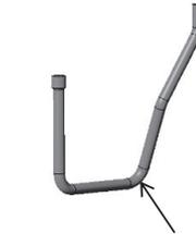
After being removed, leave the pipes at the bottom inside the unit. (Once removed from the unit, it will be difficult to re-place the pipes.)
