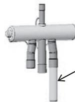
A cap for sealing the refrigerant pipe is included with the replacement kit that contains four-way valve (21S4c).
