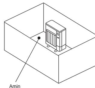
B) Install in a space with a depression height of 0.125 [m] or less.
