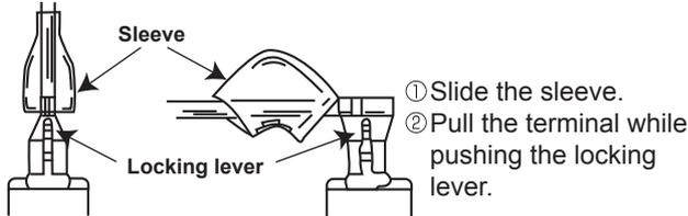
(2) The terminal with the connector shown below has the locking mechanism.
