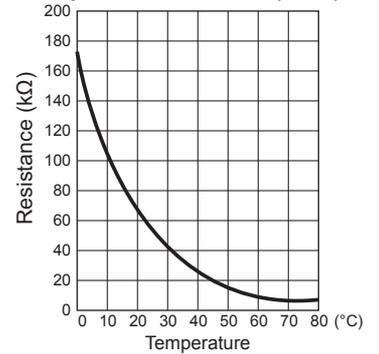
Thermistor  $R_{50} = 17 \text{ k}\Omega \pm 2\%$
