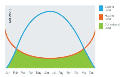
Chillers that are able to provide simultaneous heating and cooling during these periods of coincidental load, provide significant reductions in energy usage and running costs.
