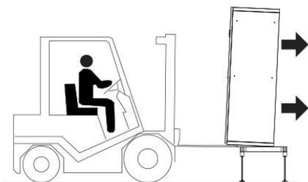
Place the machine on the frame.
