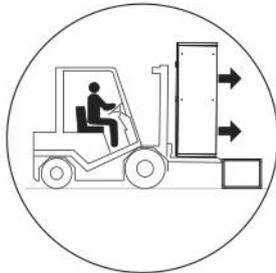
Place the machine on the plenum
