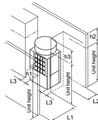
Add the dimension that exceeds the height limit (shown as "h1" through "h3" in the figures) to L1, L2, and L3 as shown in the table below.
