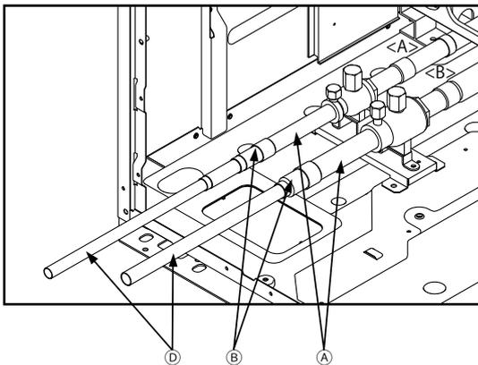
(2) When routing the pipes through the bottom of the unit
