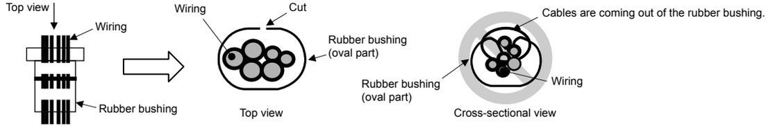
\*2 When threading the wiring through the rubber bushing, make sure the rubber bushing will not come off the sheet metal on the control box.
