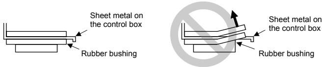
\*3 When tying the supplied tie band around the rubber bushing, make sure to leave no gap between the ends.
