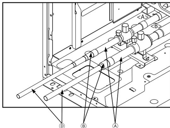
(2) When routing the pipes through the bottom of the unit
