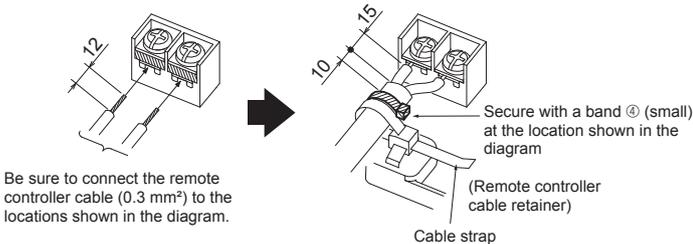
Be sure to connect the remote controller cable (0.3 mm<sup>2</sup>) to the locations shown in the diagram.
