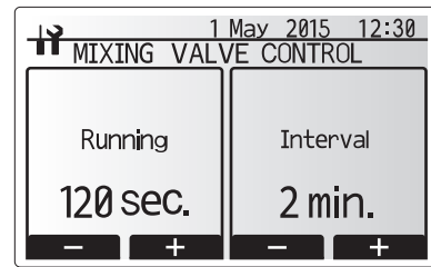
Mixing valve setting screen
