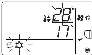
While the cooling preset temperature display blinks, pressing the button increases the cooling preset temperature, and pressing the button decreases the cooling preset temperature.
