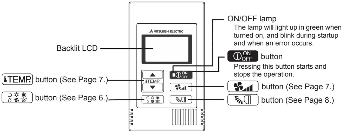
\* To set the functions that are not available on this controller (PAC-YT52CRA) such as Louver, use MA remote controller or the centralized controller.
