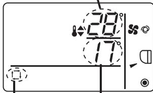
Current preset temperature (cooling/heating) appears.
