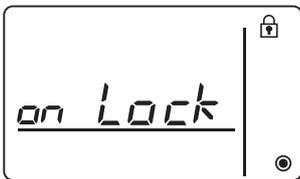
B. While the operation lock is enabled.
