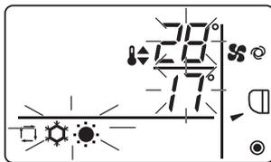
While the preset temperature (cooling/heating) display blinks, pressing the button increases the preset temperatures for both cooling and heating, and pressing the button decreases the preset temperatures for both cooling and heating.
