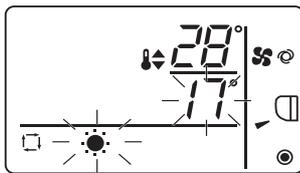
While the heating preset temperature display blinks, pressing the button increases the heating preset temperature, and pressing the button decreases the heating preset temperature.
