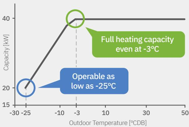
The technology behind this is an injection circuit which provides optimum amount of refrigerant to the system via a compressor through a specially designed injection port to ensure a particularly stable operation.
