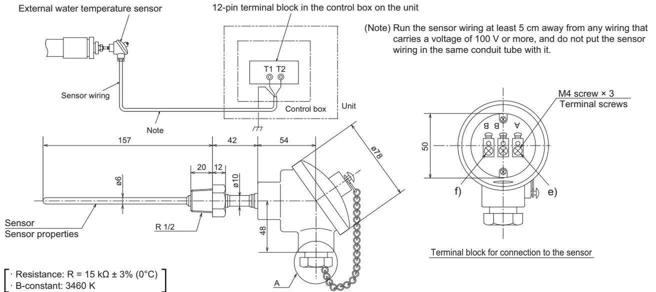
Connect the sensor wiring to terminals T1 and T2 of the 12-pin terminal block in the control box on the unit.
