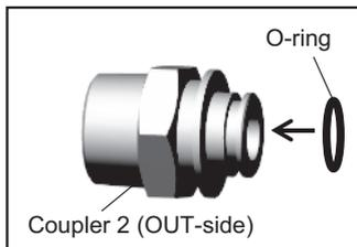
Both of the parts shown at left have a groove on the smaller end. Apply grease to the O-rings, and then fit them into the groove.
