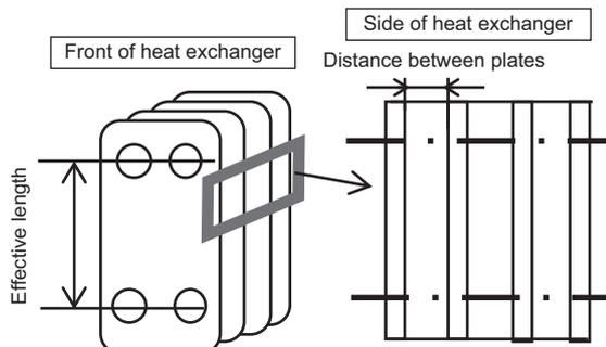
A shearing stress of 16 Pa or higher is required to reduce the amount of scale that adheres.
