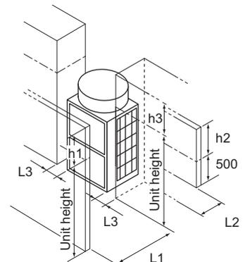
Add the dimension that exceeds the height limit (shown as "h1" through "h3" in the figures) to L1, L2, and L3 as shown in the table below.
