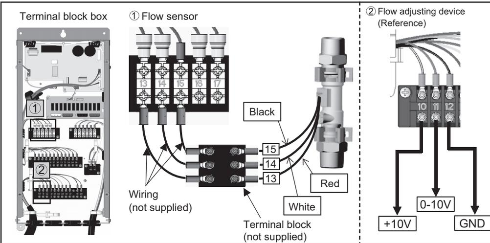
Connect the flow sensor wiring to the terminal block inside the BOX. The numbers on the wirings correspond to the numbers on the terminal block. Connect each wiring to the correct terminal. When done, hold the excess wiring with the supplied cable tie (long). Also, hold the wirings in place with a cable tie (long) where indicated as B in the figure to keep them out of contact with the pipes and other components.
