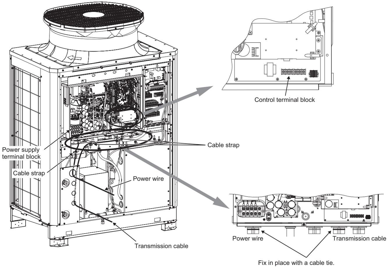
**Important:** Power supply cables larger than 25 mm<sup>2</sup> in diameter are not connectable to the power supply terminal block (TB2). Use a pull box to connect them.
