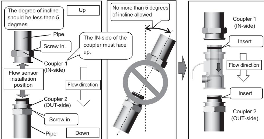
Attach the coupler to the pipe so that **the IN-side of the coupler faces up and the OUT-side of the coupler faces down. (Water flows from top to bottom.) The incline of the pipe should not exceed 5 degrees.**
