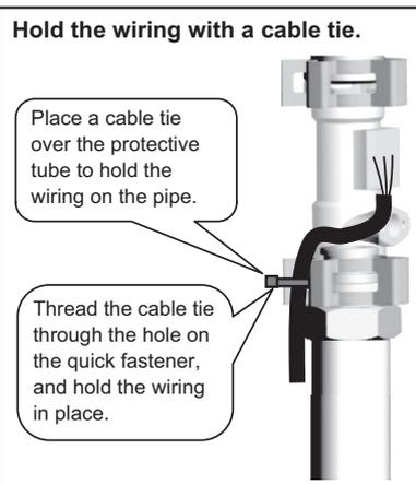
Insert the flow sensor into the couplers, and then fit the quick fasteners where the flow sensor and the couplers are connected to each other. Keep the quick fasteners out of contact with the wiring so as not to damage the wiring. Hold the wiring to the quick fastener with a (short) cable tie as shown in the figure to keep the wiring from being damaged.
