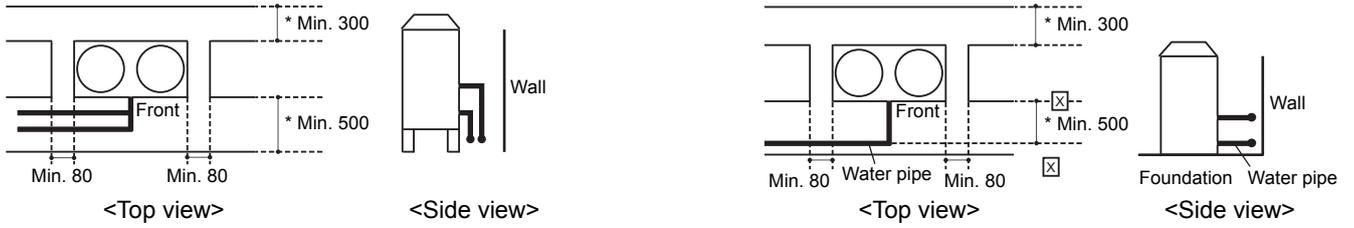
Leave a space of at least 500 between the unit and the water pipe if it is not possible to install the unit on a raised foundation. (See ☒ in the figure.)
