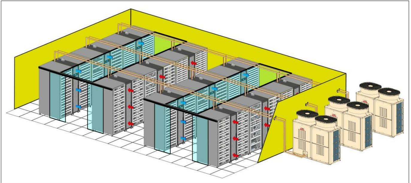
The cold aisle containment allows maximum energy savings and an optimum distribution of the air flow. The arrangement of the indoor units – one unit for each row of racks – ensures continuity of operation in case of failure of a system.
