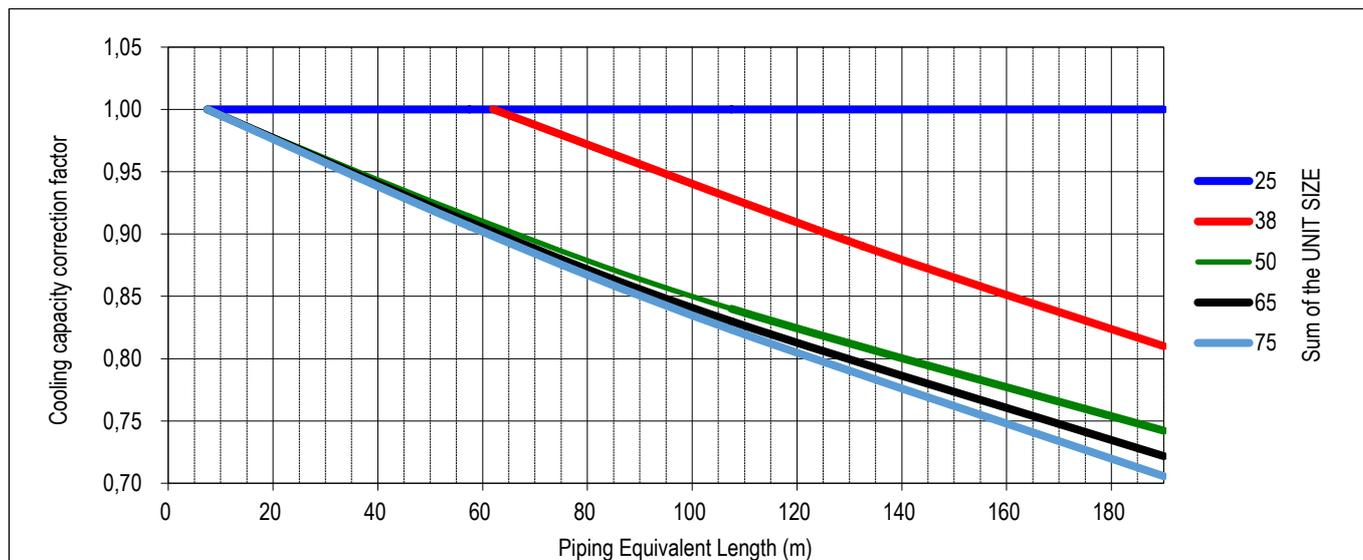
Piping Equivalent length = (Actual piping length to the farthest indoor unit) + (0.50 x number of bends in the piping) m.
