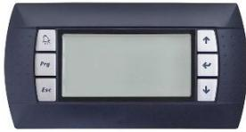
The microprocessor control system is equipped with 6-key terminal and backlit graphic display on which all information in different languages or easily identifiable symbols are displayed. The system disposes of a "flash" memory that preserves the information even in absence of power supply. Part of memory is dedicated to the registration of intervened events - up to 100 events.
