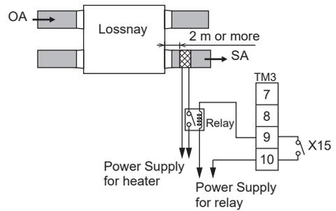
**<Examples of electric wiring for function setting No.58 TM3 7-10>**
