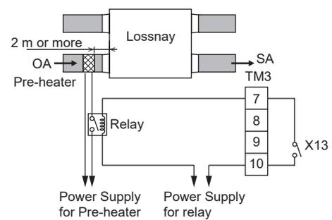
**<Examples of electric wiring for function setting No.81 TM3 8-10>**
