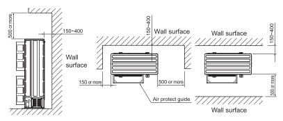
(2) Multiple unit installation: \* Installation of multiple units in series must be no more than five units.
