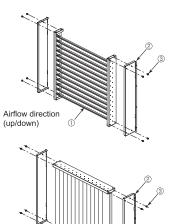
(2) Fix the air outlet guide ① assembled in (1) to the unit with the attachment screws 3 (at the 8 points)
