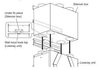
Fix the Silencer box with the two (P-250/350SB-E) or four (P-500SB-E) screws.
