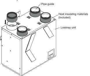
2) Apply a good amount of a caulking material (liberally) to the pipe guides and heat insulating materials. Insufficient application may cause water leakage and air leakage.
