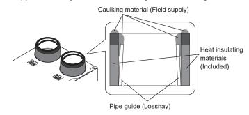
3) Place the Silencer box while aligning the position of the connection ports at the bottom of the Silencer box with the pipe guides of the Lossnay unit. Make sure that the under fix piece of the Silencer box touches the wall mount hook top of the Lossnay unit.
