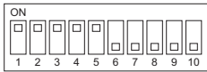
The figure at left shows that the switches 1 through 5 are set to ON and 6 through 10 are set to OFF.
