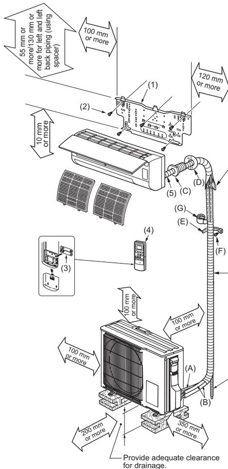
Be sure to use wall hole sleeve (C) to prevent indoor/outdoor connecting wire (A) from contacting metal parts in the wall and to prevent damage by rodents in case the wall is hollow.
