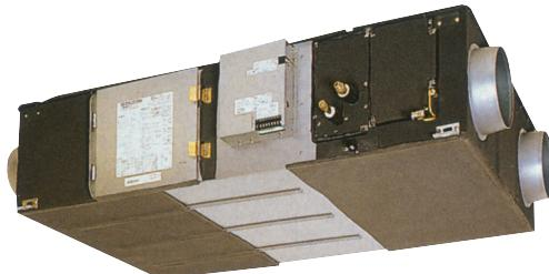
The **GUF-RD4** fresh air processing units combine a Lossnay Mechanical Ventilation with Heat Recovery (MVHR) unit with a DX coil connectable to a VRF system, to heat and cool the supply air delivered to the space. The combination of these technologies provides effective tempering of fresh air entering commercial spaces, taking the load off other cooling/heating services, and eliminating any chance of draughts.
