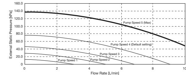
The performance showing in the graph includes pressure drop of both cylinder unit and outdoor unit. Before installation, please check if the maximum performance of water circulation pump 1 can accommodate the per user drop of external heating circuit.
