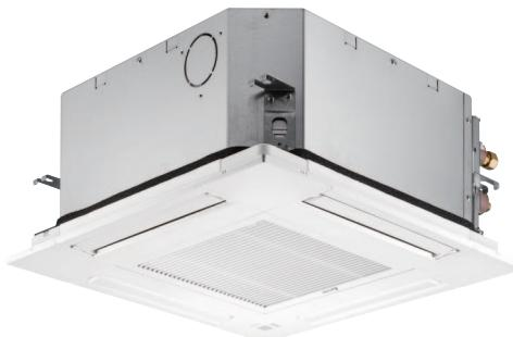
The **PLFY-WL-VFM-E** ceiling cassette unit connects to the Hybrid Branch Controller and uses water as the heat transfer medium. Providing a smart air conditioning solution for tight ceiling spaces, and designed to fit directly into standard 600mm square ceiling grids, these units are a perfect choice for both offices and retail applications. The optional 3D i-see sensor grille optimises both energy consumption and comfort levels.
