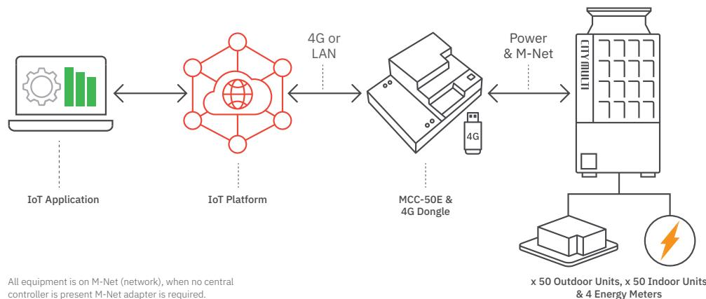
All equipment is on M-Net (network), when no central controller is present M-Net adapter is required.
