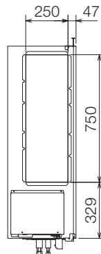
An inspection opening is required for installation and regular maintenance (check) of the drain pump. When SA temp. control is selected, another inspection opening may be required in front of the unit for SA thermistor replacement only when an error occurred on the SA thermistor.
