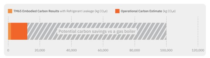
Operational carbon data for heating requirements, according to heat pump ErP fiche at medium temperature (55°C), average climate conditions and equivalent boiler heat output. Gas boiler assumptions: embodied carbon of 300kg CO<sub>2</sub>e, efficiency of 93%, service life of 15 years.
