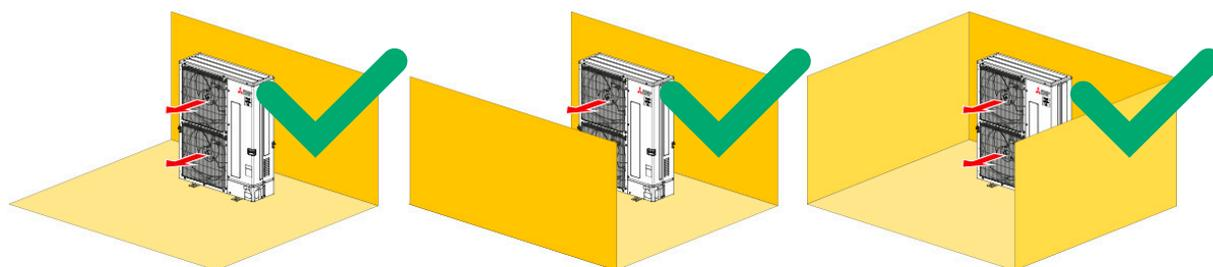
DO NOT INSTALL THE OUTDOOR UNIT IN A SEMIBASEMENT, BASEMENT OR MACHINERY ROOM WHERE THE REFRIGERANT REMAINS IN THE ROOM WHEN IT LEAKS OUT.
