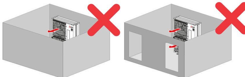
Do not install in semibasement, basement or machinery room
