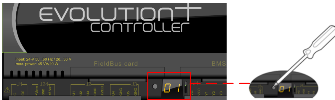
7 segment display for the addressing procedure using the hardware
