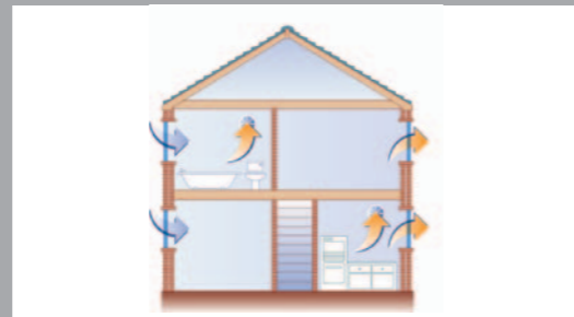
Background ventilators and intermittent extractor fans
