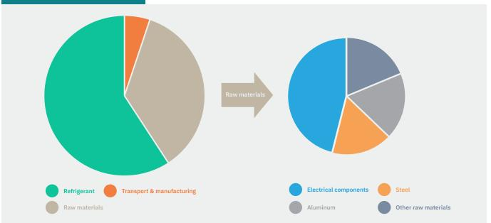
We see that a large contributor to embodied carbon in MEP are the small electrical components and printed circuit boards. These components have a high concentration of exotic metals and plastics and carbon intensive manufacturing processes resulting in a high carbon footprint. It is difficult for manufacturers to reduce embodied carbon by focussing on these elements.
