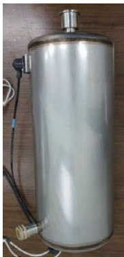
Photo 16-14-3 Booster heater without insulation
