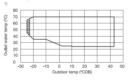
Outdoor temp. -25°CDB/Outlet water temp. 45~65°C Outdoor temp. -20°CDB/Outlet water temp. 35~70°C Outdoor temp. 43°CDB/Outlet water temp. 24~70°C
