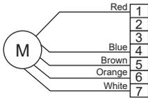
Measure the resistance between the connector pins with a multimeter (at the ambient temperature 20°C [68°F]).
