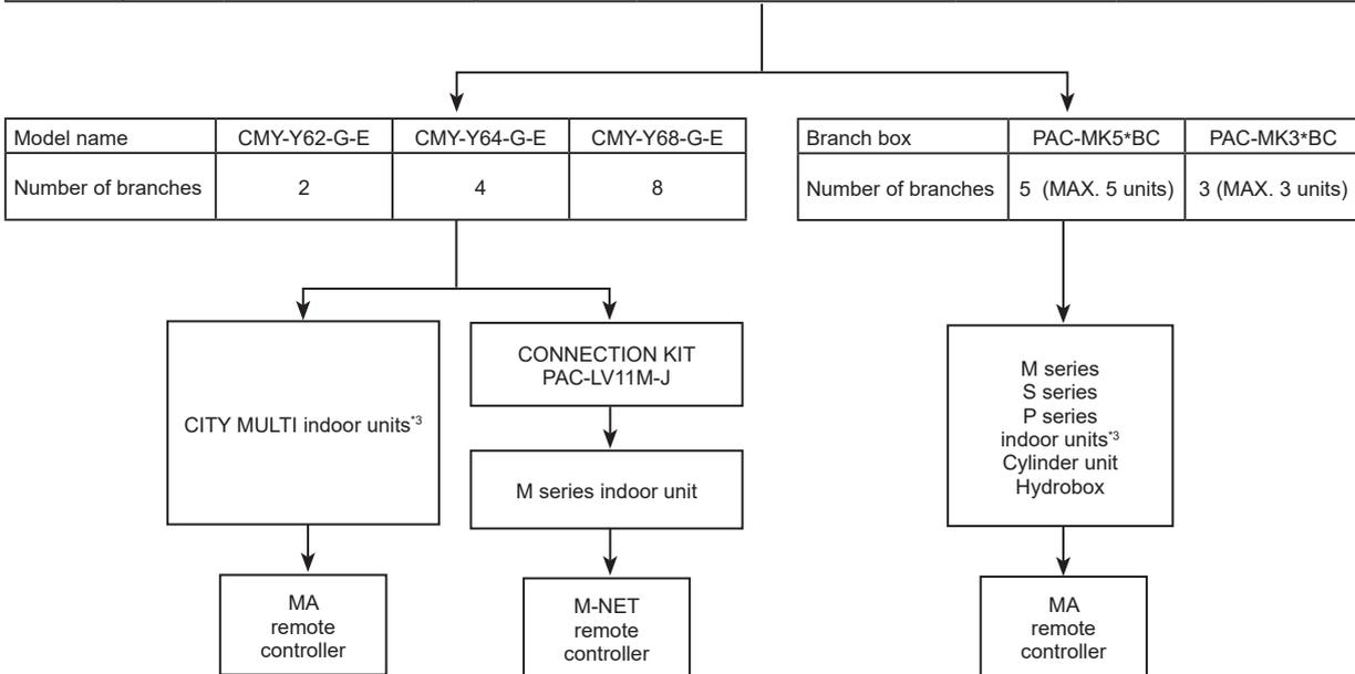
\*1. When connecting ecodan unit, the total capacity of connected Air to Air indoor units is up to 130% of the outdoor unit (Air to Air 130% + ecodan). However, when operating Air to Air indoor unit(s) in heating mode and ecodan unit in DHW or heating mode at the same time, the maximum connectable Air to Air indoor unit is below.
