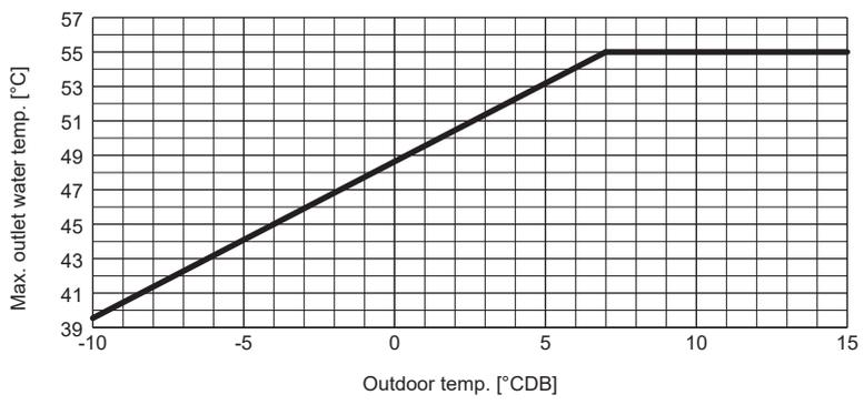
**3-4-3-1. Temperature curve of max. outlet water**
