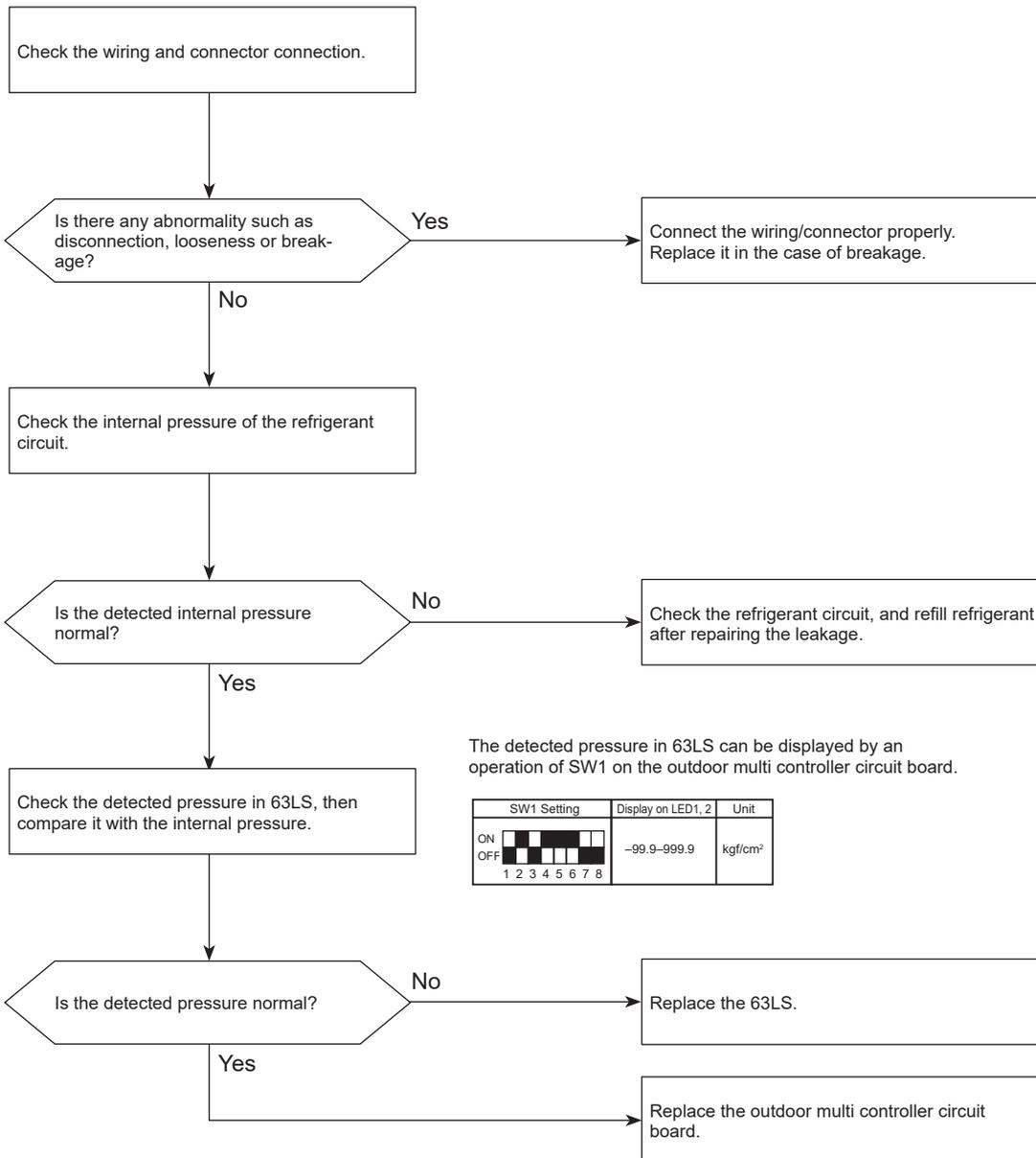
The detected pressure in 63LS can be displayed by an operation of SW1 on the outdoor multi controller circuit board.
