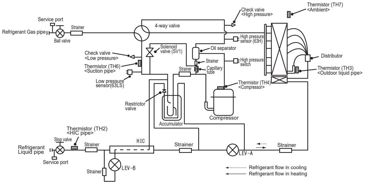
Capillary tube for oil separator:  $\varnothing 2.5 \times \varnothing 0.8 \times L1000$
