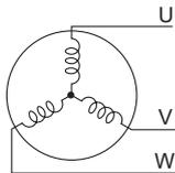
Measure the resistance between the terminals with a multimeter (at the ambient temperature 20°C [68°F]).
