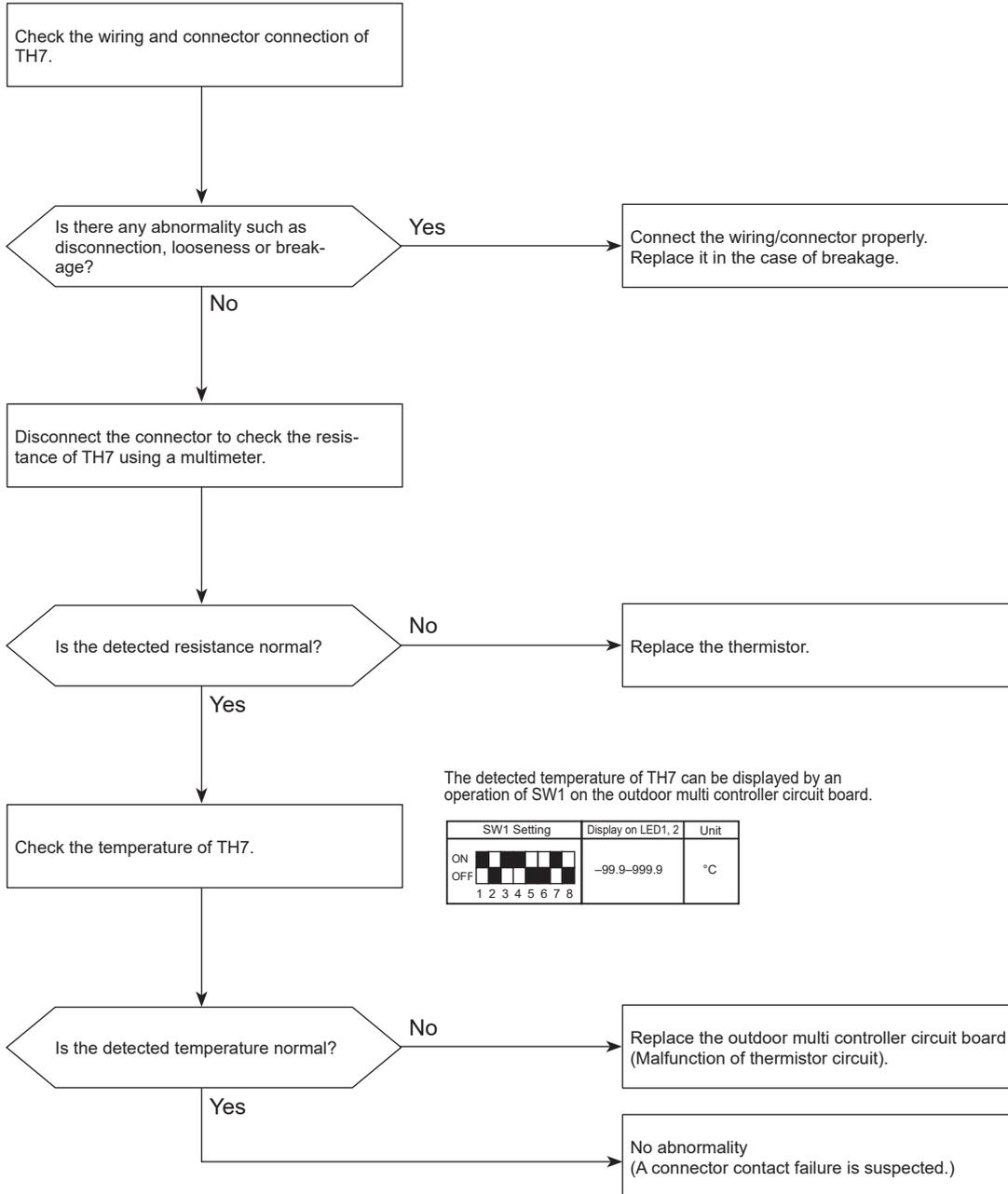
The detected temperature of TH7 can be displayed by an operation of SW1 on the outdoor multi controller circuit board.
