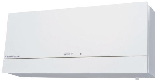
The **VL-100** wall mounted Lossnay supplies fresh air into a room, simultaneously extracting stale air in an energy efficient manner. The recovery of both latent heat and sensible heat ensures a comfortable internal environment, minimising heat loss and saving both energy and costs. Easy to install, this compact unit is ideal for single room applications, such as small offices, bedrooms, and spaces where a ducted system is not an option.
