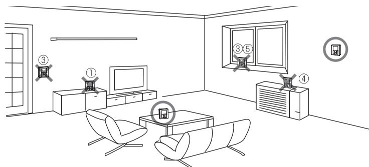
A room sensor is incorporated in each wireless remote controller. So wireless remote controller is placed in an improper location, the desired temperature may not be obtained.
