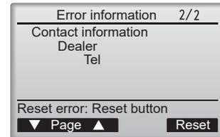
2. Press the **F4** button or the
