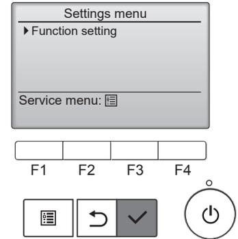
2. Set the indoor unit refrigerant addresses and unit numbers with the [ F1 ] through [ F4 ] buttons, and then press the [ ✓ ] button to confirm the current setting.
