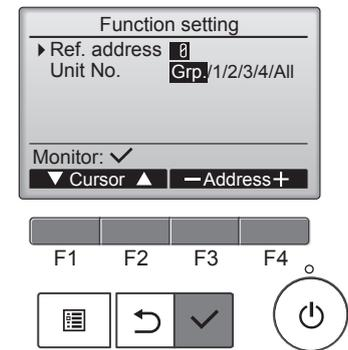
3. When data collection from the indoor units is completed, the current settings appears highlighted. Non-highlighted items indicate that no function settings are made. Screen appearance varies depending on the "Unit No." setting.
