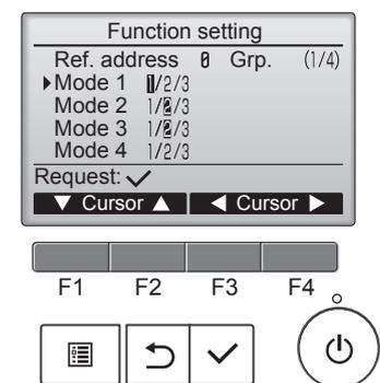
5. When the settings are completed, press the [ ✓ ] button to send the setting data from the remote controller to the indoor units. When the transmission is successfully completed, the screen will return to the Function setting screen.
