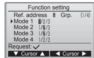
4. Use the [ F1 ] or [ F2 ] button to move the cursor to select the mode number, and change the setting number with the [ F3 ] or [ F4 ] button.
