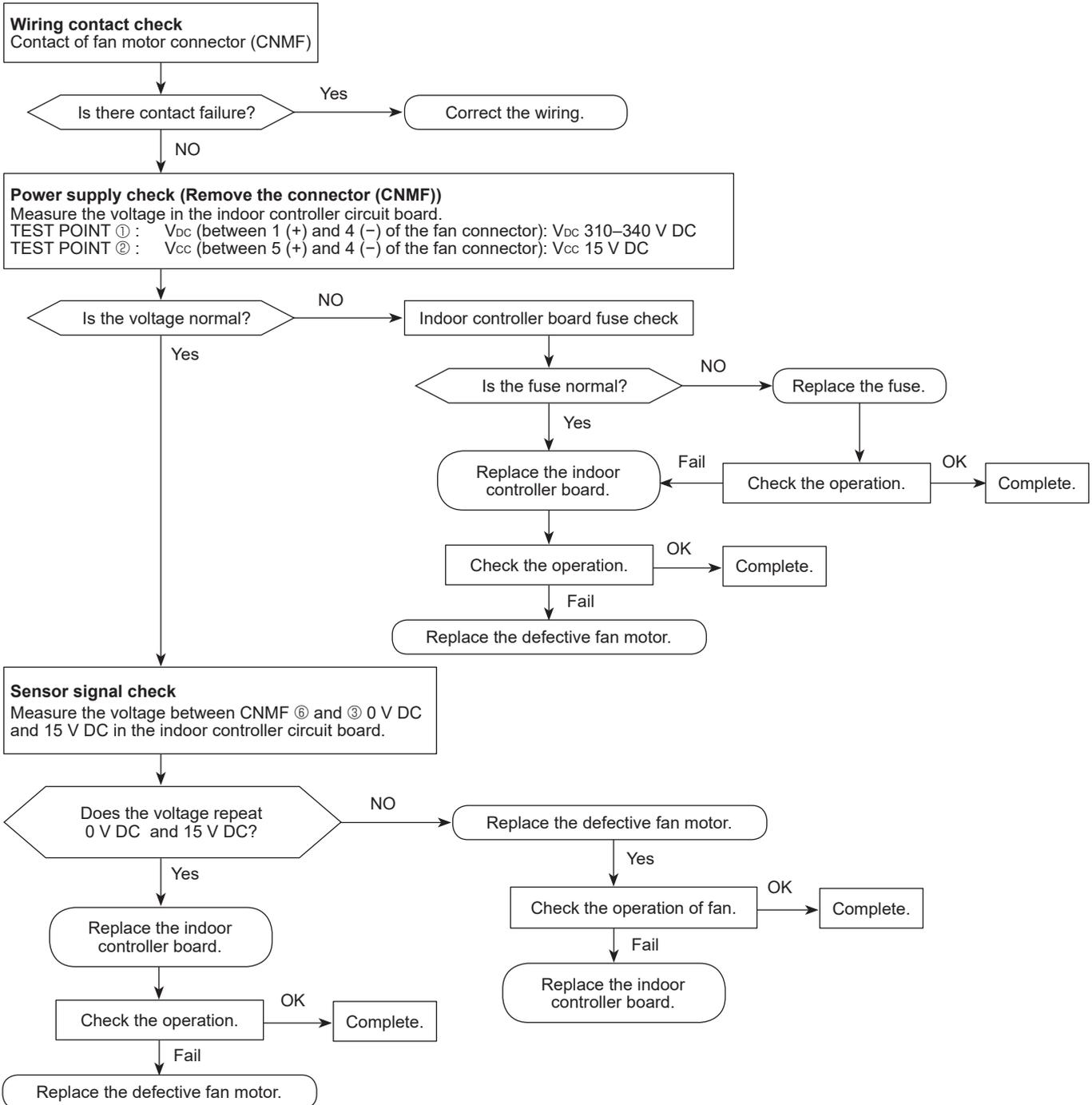
Symptom: The fan motor does not stop when pressing the stop button on the remote controller.
