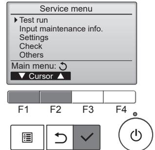
2. Select "Test run" with the [ F1 ] or [ F2 ] button, and press the [ ✓ ] button.
