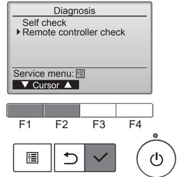
2. Select "Remote controller check" from the Diagnosis menu, and press the [ ✓ ] button to start the remote controller check and see the check results.
