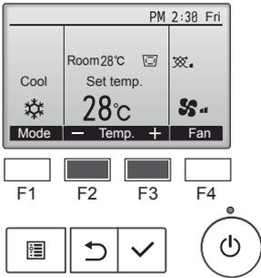
Press the [F2] button to decrease the preset temperature, and press the [F3] button to increase.
