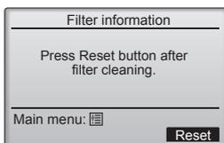
Press the [F4] button to reset filter sign. Refer to the indoor unit Operation Manual for how to clean the filter.
