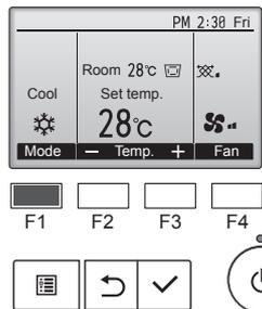
Press the [F1] button to go through the operation modes in the order of "Cool", "Dry", "Fan", "Auto", and "Heat". Select the desired operation mode.
