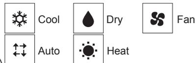
• Operation modes that are not available to the connected outdoor unit models will not appear on the display.
