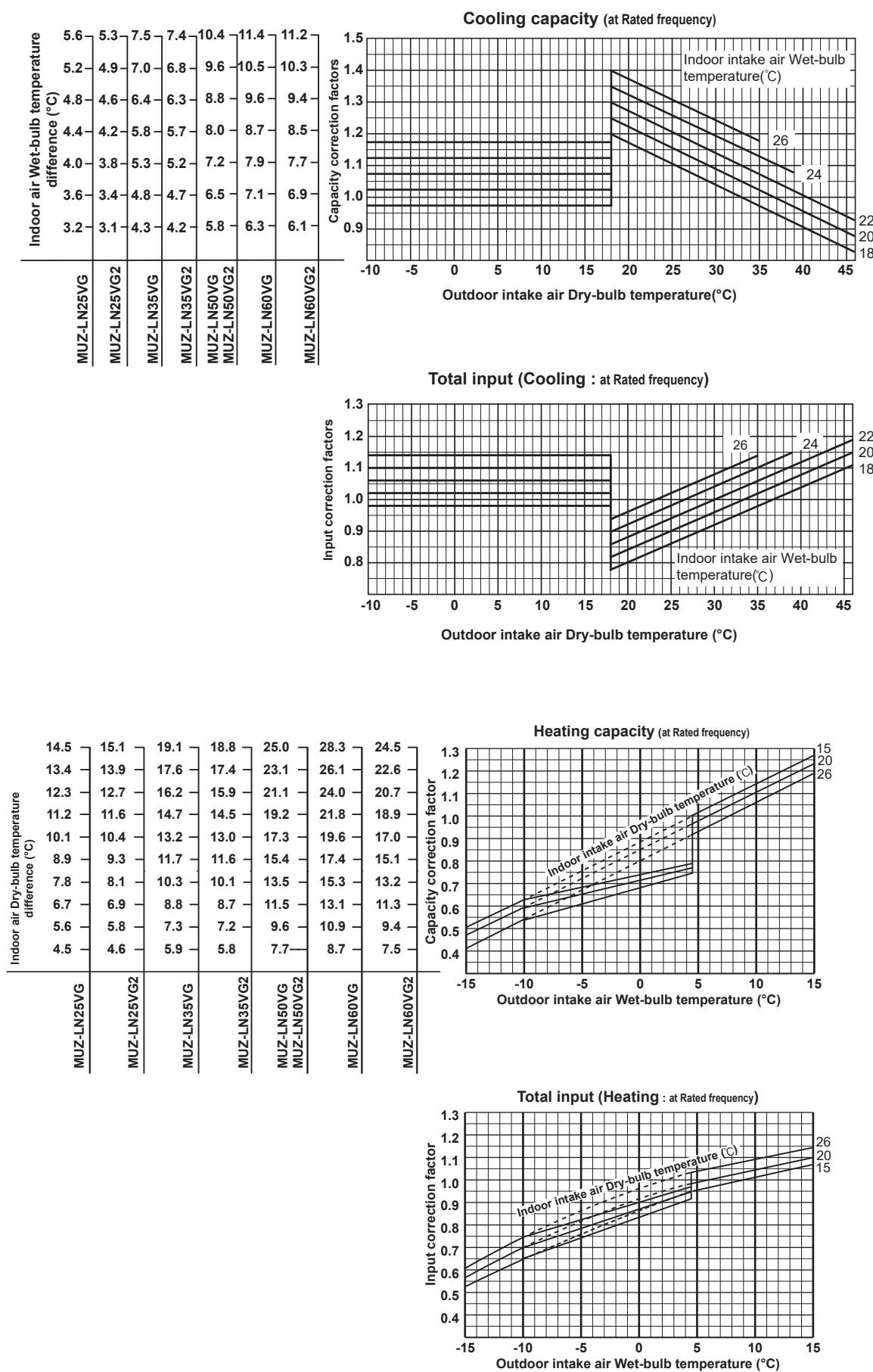
NOTE: The above broken lines are for the heating operation without any frost and defrost operation.
